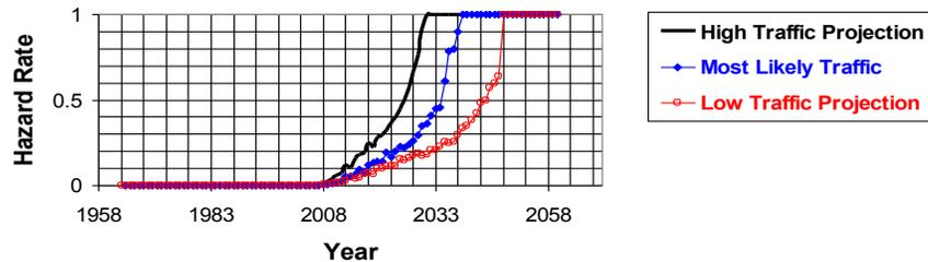
Time dependant failure Probabilities of components
