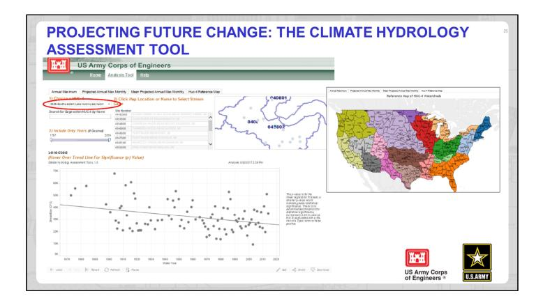
The front page of the CHAT tool allows the user to select a gage from the pulldown menu or by searching by name. It also shows the HUC-4 watershed map and a simple linear regression of observed past annual peak streamflows for context
